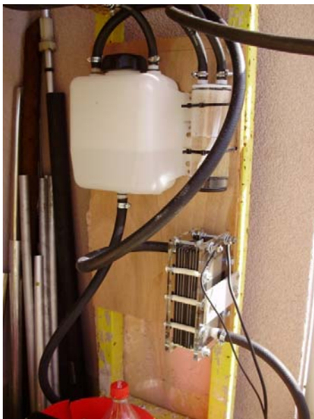
Fig. 3. Trgomar H 2 O Maxpower SS1 setup
